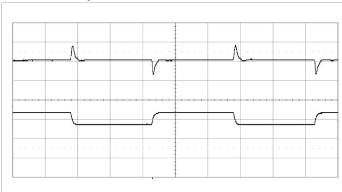
Output voltage response to load current step change (1.5–4.5–1.5 A) at V_i = 12\text{ V} , C_o = 3 \times 100\ \mu\text{F} + 270\ \mu\text{F}/10\text{m}\Omega . Default compensation settings. Scale: 50 mV/div, 5 A/div, 100 \mu\text{s} /div.
